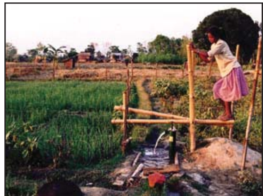
The Bamboo Treadle Pump allows poor farmers to access groundwater during the dry season. The treadles and support structure are made of inexpensive, locally available materials and the pump can be manufactured locally by metalworking shops. (Designer: Gunnar Barnes of Rangpur/Dinajpur Rural Service and International Development Enterprises [IDE] Nepal)
