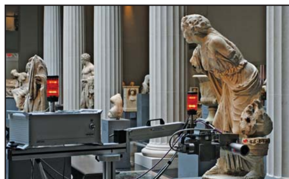
X-ray fluorescence spectroscopy is used by Metropolitan Museum of Art scientists to investigate the original polychromy of a Roman sculpture (Schulz, 2009)
